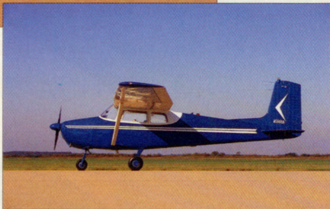
N1655H is an S model equipped with a 180-horsepower Lycoming IO-360 engine (above). N5000A is the first "true" 172, built in 1955 as a 1956 model (left).
